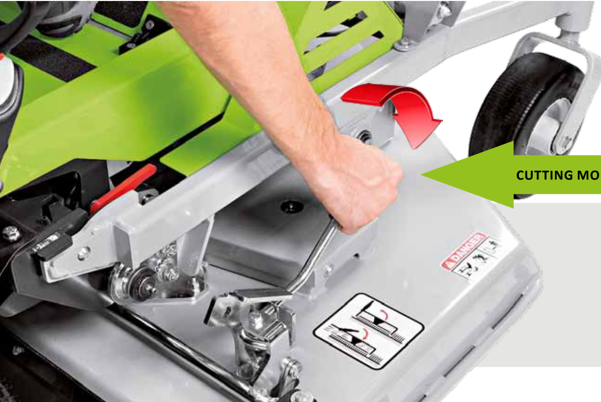
A REAR DISCHARGE MODE CUTTING CHAMBER OPEN
