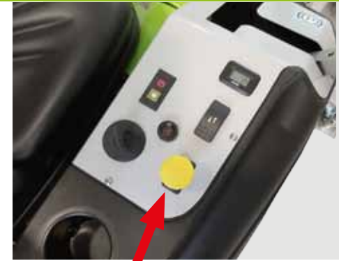
Electromagnetic clutch for blade engagement.
